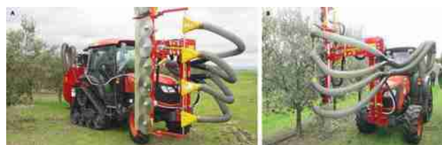
Fig. 2 - A) Cutting bar equipped with the selective pruning device; B) The pruning machine working along a row.
